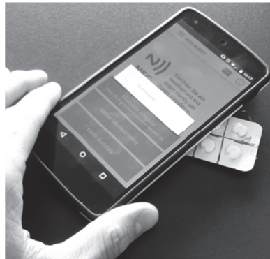
Figure 1: NFC interaction of application and intelligent blister
